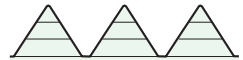
利用切削丝锥加工的内螺纹 Female thread cut by a cutting Tap
