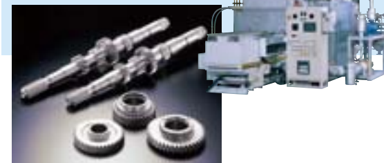
Vacuum carburizing of transmission gears.
