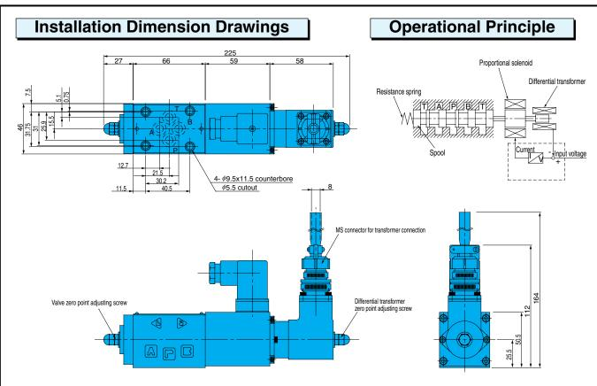
The gasket mounting method conforms to ISO4401-AB-03-4-A.
