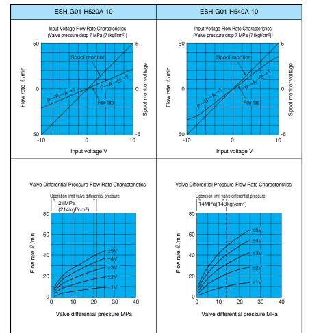
Note)  $\pm$ 10V input amp factory default data. Rotating the GAIN trimmer clockwise (rightward) increases the flow rate by up to 10%.
