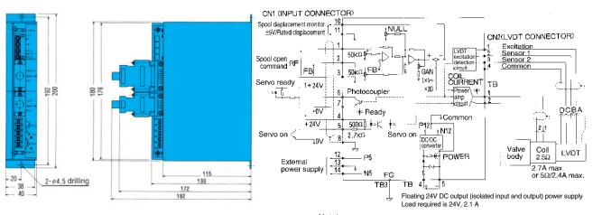
Note) Since G03, G04, and G05 are pilot operation types, there is an LVDT on the main spool, but connection is identical.
